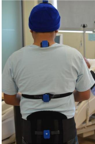
Figure 2. IMU sensor orientation on nurse during experiment
