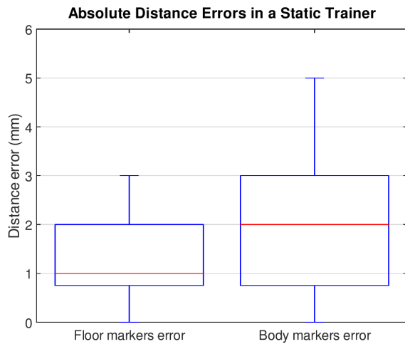
Fig. 12. Boxplot of the resulting differences between the Gold Standard and the Floor Markers (left) and Body Markers (right) protocols for absolute distance variables in a static trainer.
