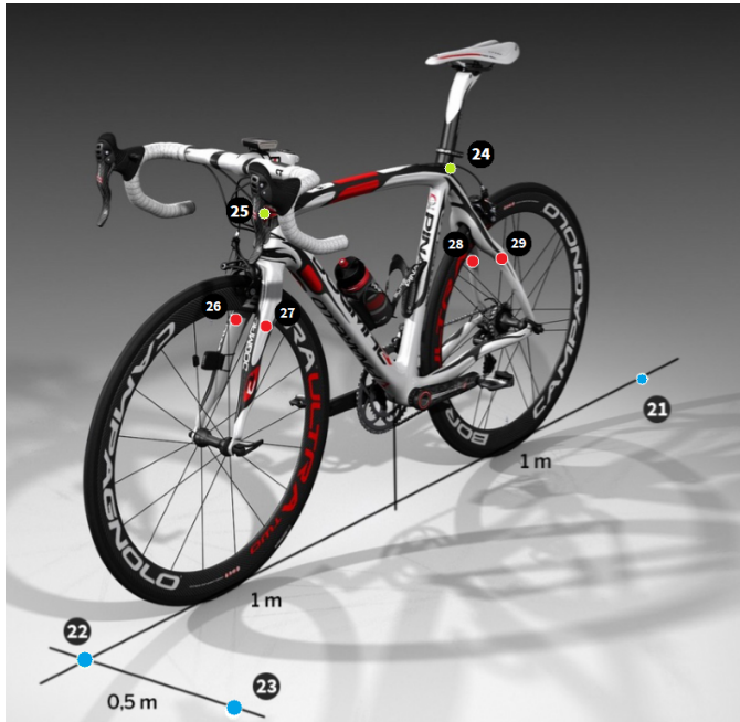
Fig. 3. Bike markersets used for the captures. In blue: floor markers. In green: simplified bike markers. In red: complete bike markers.
